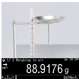
First measure the empty weight.
